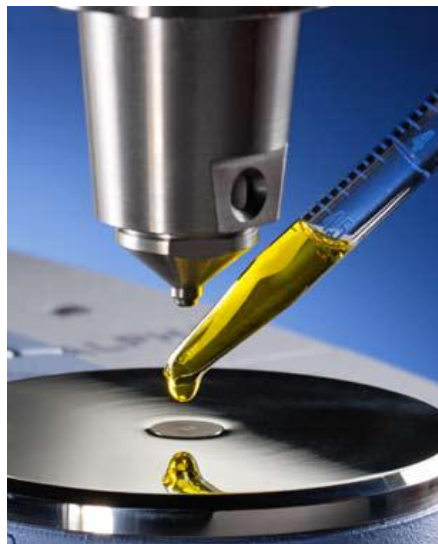
Figure 4. Diamond ATR accessory in Bruker Optics' ALPHA.
